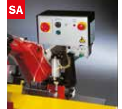
Discesa controllata Gravity down feed
