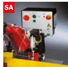
Discesa controllata Gravity down feed
